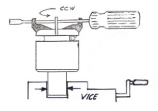
2. Demount the inserts from the fingers. Set up Grippex in a vice and clamp on the shank. Use a screwdriver and turn the body ccw and the body will be loosen from the shank.
