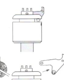
4. Unscrew the three screws (M4x8 mm) on the shank till the cylindrical pins can pass and be put aside.
