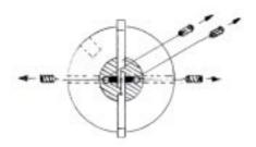
2. Unscrew the two screws on the body and the two stop-screws on the front of the shaft.
