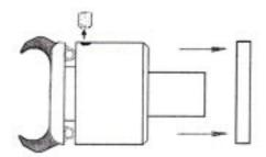
1. Unscrew the Valve-screw and remove the cover.
