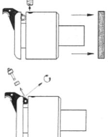
1. Unscrew the Valve-screw and remove the cover.
