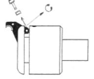
2. Dismount the locking washer on one side of the finger and push the roller pin out of the finger.
